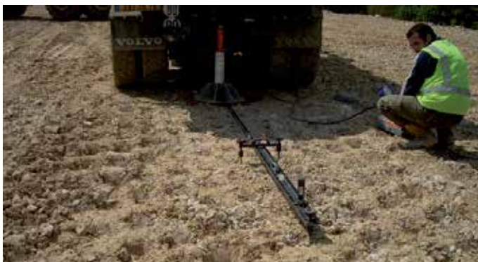
Figure 18: Measurement of the degree of compaction
