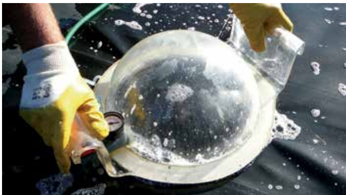
Figure 40: Quality control with vacuum chamber
