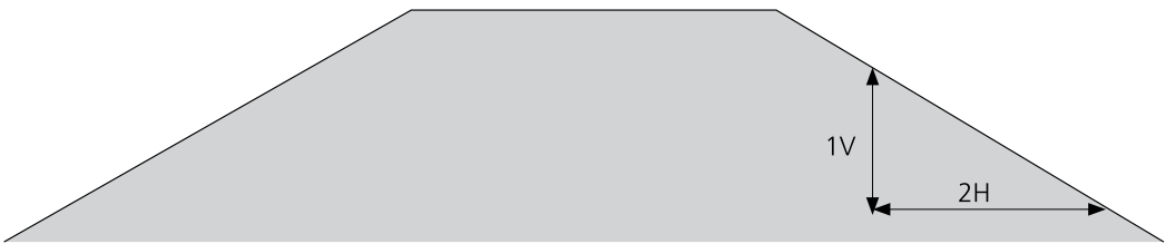
Figure 23: Example of a 1V/2H slope
