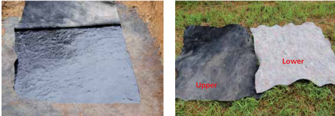
Figure 14: EPDM geomembrane and colour difference between the upper and lower geotextile
