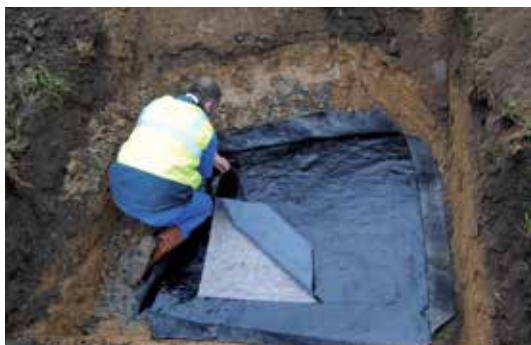
Figure 12: Taking samples of the EPDM geomembrane
