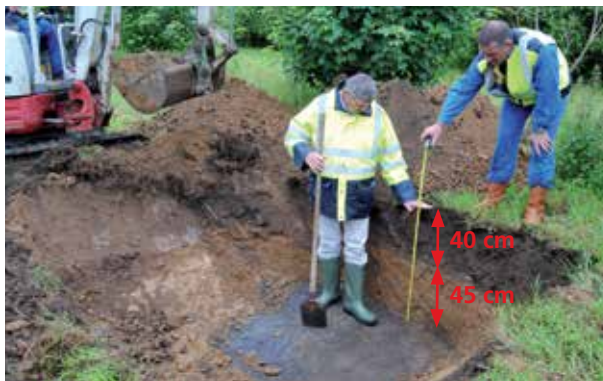
Figure 15: Top of the mound – Cross section of the soil cover and condition of the upper protective geotextile
